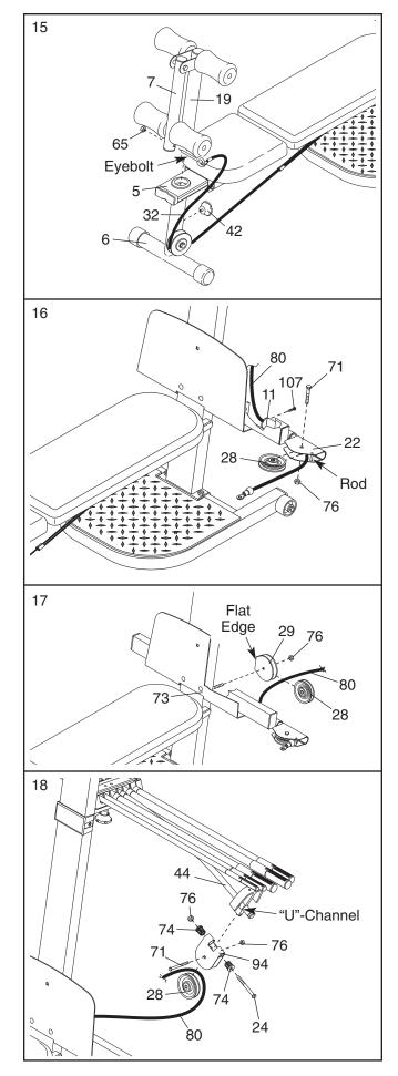
Wrap the Long Cable (80) under a 90mm Pulley (28) as shown. Attach the Pulley and a Pulley Guard (29) to the Upright (3) with an M10 x 113mm Button Head Bolt (40) and an M10 Nylon Locknut (76). Make sure the flat edge of the Pulley Guard is on the bottom.
